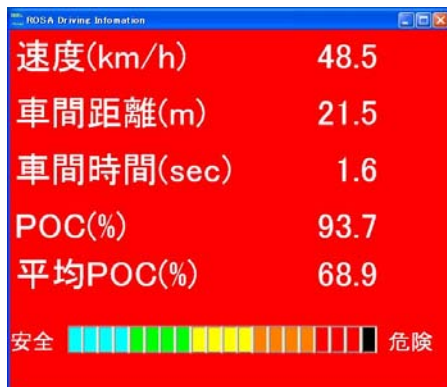
Figure 3. Screen of the monitor mounted on the vehicle while driving. Labels are velocity(km/h), following distance (m), time gap (sec), current POC, mean POC and an indicator of current POC.
