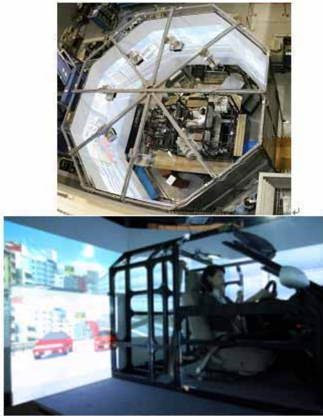
Fig. 1 Omni-directional Visual System
