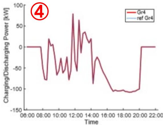
Not provide enough discharging power in order to keep and satisfy the terminal SoC constraint.
