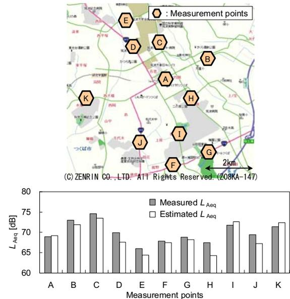
Figure 9. Comparison between estimated and measured  $L_{Aeq}$
