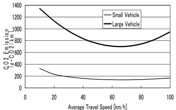
Figure 3. CO<sub>2</sub> Emission Model used in the study
