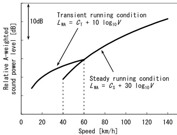
Figure 2. Road vehicles' sound power calculation model of ASJ RTN-Model 2003<sup>[11]</sup>
