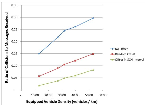
Figure 5: Impact of Scheduling Approaches on the Ratio of Collisions to Messages Received for Single-Band Radios
