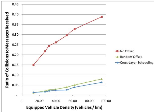
Figure 6: Impact of Scheduling Approaches on the Ratio of Collisions to Messages Received for Multi-Band Radios
