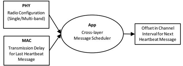
Figure 4: Data Flow Diagram for Cross-Layer Message Scheduling
