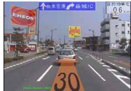
Fig. 10. Superimposing results of virtual navigation information onto real images
