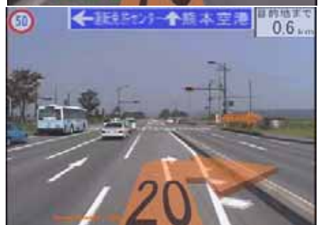
Fig. 13. Output of refined VICNAS system
