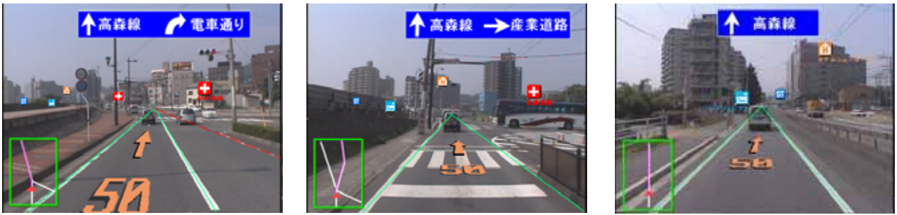
Fig. 10. Superimposing results of virtual navigation information onto real images
