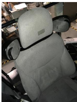
Fig. 2 Driving simulator equipped with the left and right headrest-speakers.
