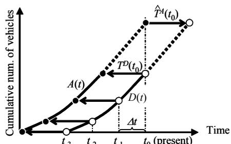
Fig. 4 Travel time prediction using cumulative flow diagram.
