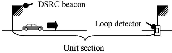
**Fig. 2 Sensor arrangement of uplink travel time prediction**
