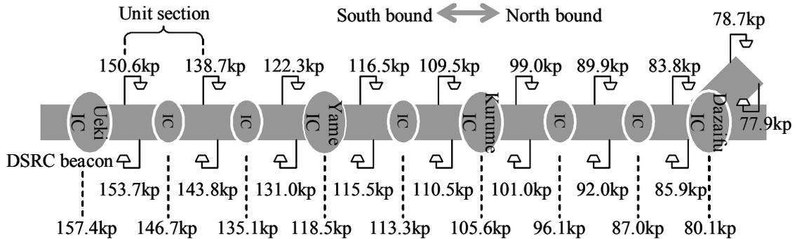
Fig. 5 Arrangement of DSRC beacons and interchanges on the Kyushu Expressway for the validation.
