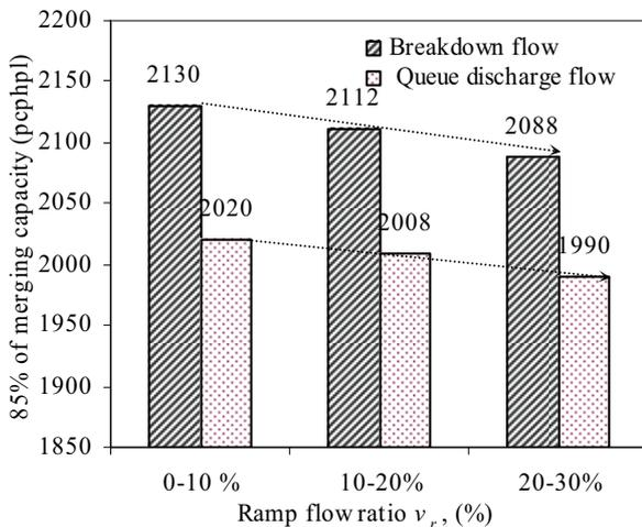
Figure 7. The 85 percentile values of merging capacity distribution at different levels of  $v_r$ .
