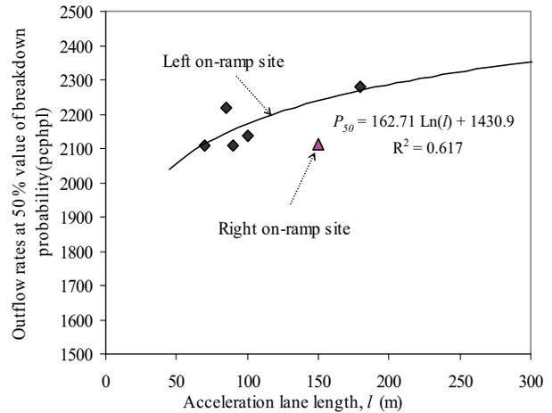
Figure 9. The relationship between  $P_{50}$  and the acceleration lane length  $l$
