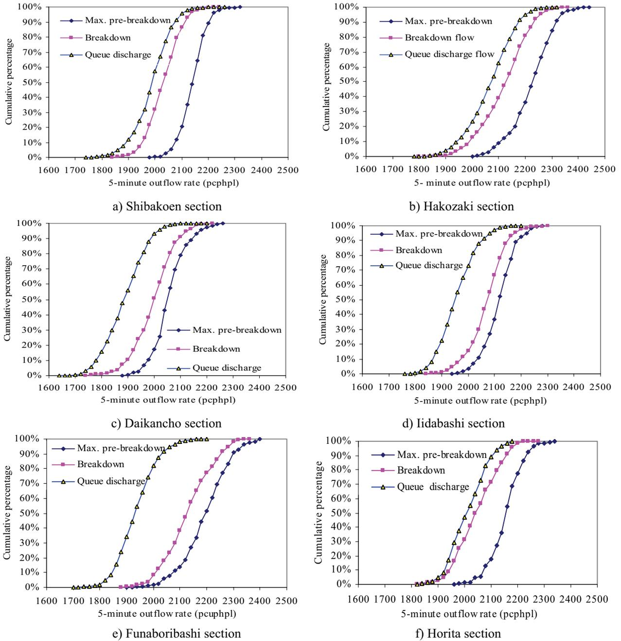
Figure 4. Observed distributions of the three aspects of merging capacity at the investigated sections
