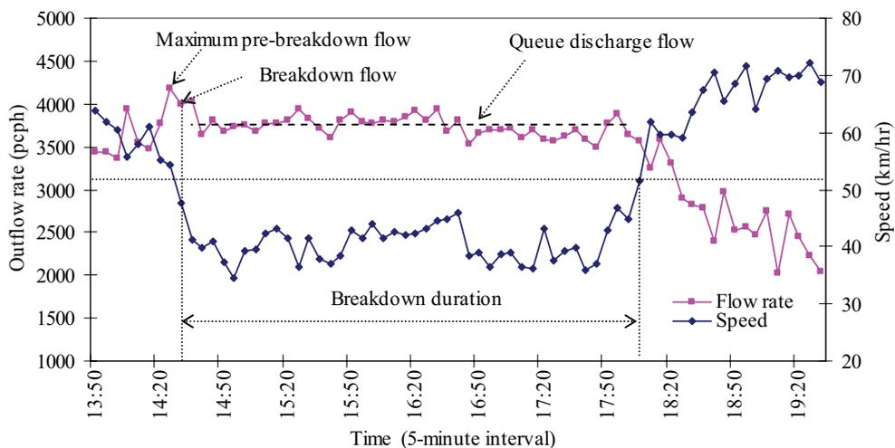
Figure 3. Example of a breakdown event observed at Shibakoen section on Jan. 28, 2005
