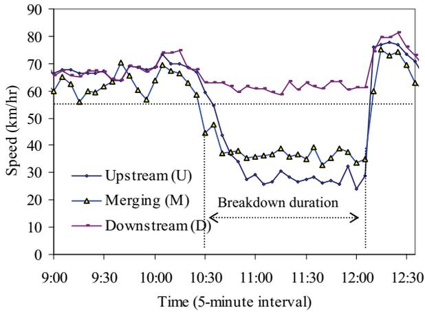
Figure 2. Speed profile of the three detectors at Iidabashi merging section
