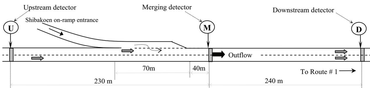
Figure 1. Detector location and layout of Shibakoen merging section (not to scale)
